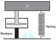
If the amplitude of free vibration response reduces from 8 mm to 1.5 mm in 3 cycles, that damping ratio of the system is \_\_\_\_\_\_. (round off to three decimal places).
