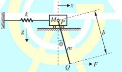
Assume that the spring deflects only horizontally and force F is applied horizontally at Q. For this system, the Lagrangian, L is
