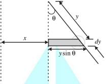
So, total displacement of rod  $= x + y \sin \theta$
