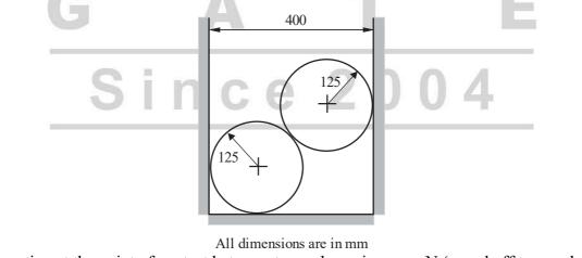
The reaction at the point of contact between two spheres is \_\_\_\_\_ N (round off to one decimal place).
