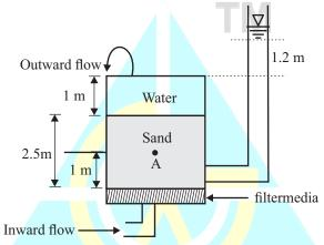
The effective stress (in kPa, round off to two decimal places) at point A, located 1 m above the base of tank, is \_\_\_\_\_.
