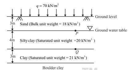
Immediately after preloading, the effective stresses (in kPa) at points P and Q respectively, are
