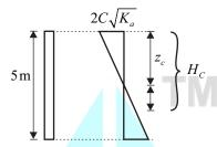
When tension crack has occurred –
