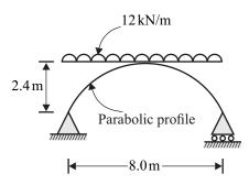
Neglecting self-weight, the maximum bending moment generated in the structure (in kN.m, round off to the nearest integer), is .
