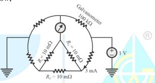
As the bridge is balanced, the reading of galvanometer will be zero.
