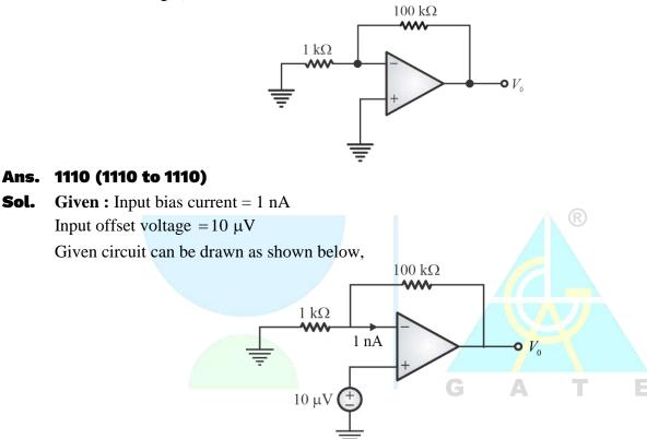
Applying KCL at inverting terminal,
