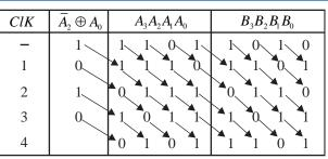
So, after four clock pulses, A = 0101 and B = 1101
