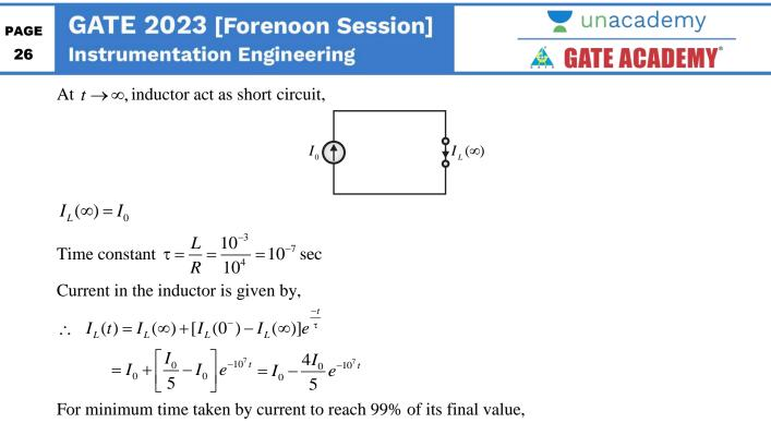
$$I_{L}(t) = 0.99I_{0} \text{ then } 0.99I_{0} = I_{0} - \frac{4I_{0}}{5}e^{-10^{7}t}$$
