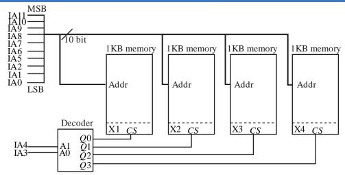
The input memory addresses (IA11–IA0), in decimal, for the starting locations (Addr=0) of each block (indicated as X1, X2, X3, X4 in the figure) are among the options given below. Which one of the following options is CORRECT?
