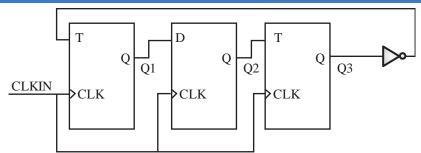
Which one of the given values of (Q1, Q2, Q3) can NEVER be obtained with this digital circuit?
