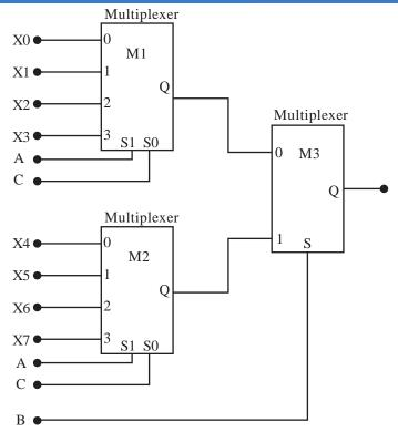
Which one of the following set of values of (X0, X1, X2, X3, X4, X5, X6, X7) will realise the Boolean function  $\bar{A} + \bar{A}.\bar{C} + A.\bar{B}.C$ ?
